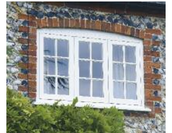
Cottage flush casement windows finished in "Off-White" featuring 22mm true bars, putty glazing and 14mm ultra slim double-glazed units.
