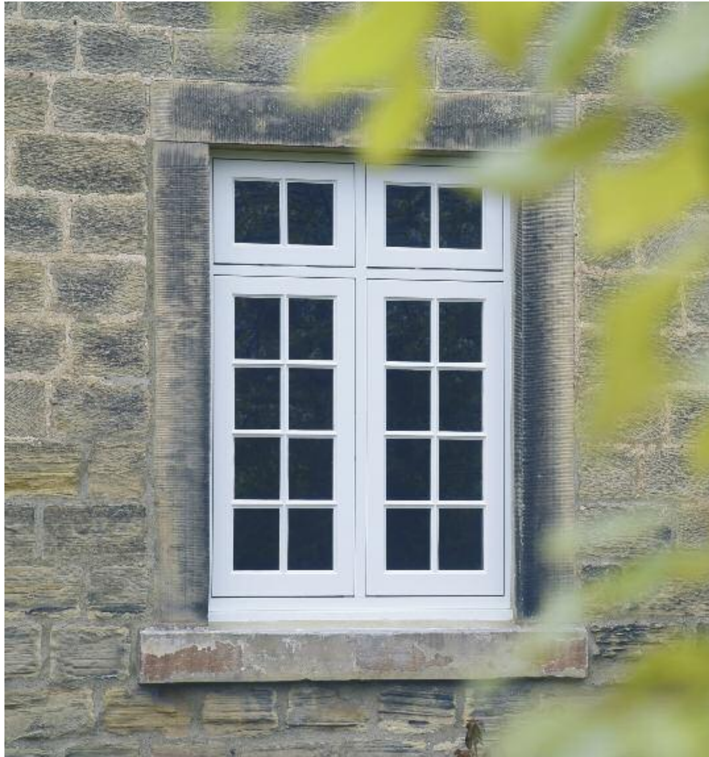
Flush casement windows finished in 'Off-White' featuring 14mm ultra-slim double-glazed units with krypton gas, along with 22mm true bars and putty glazing.
