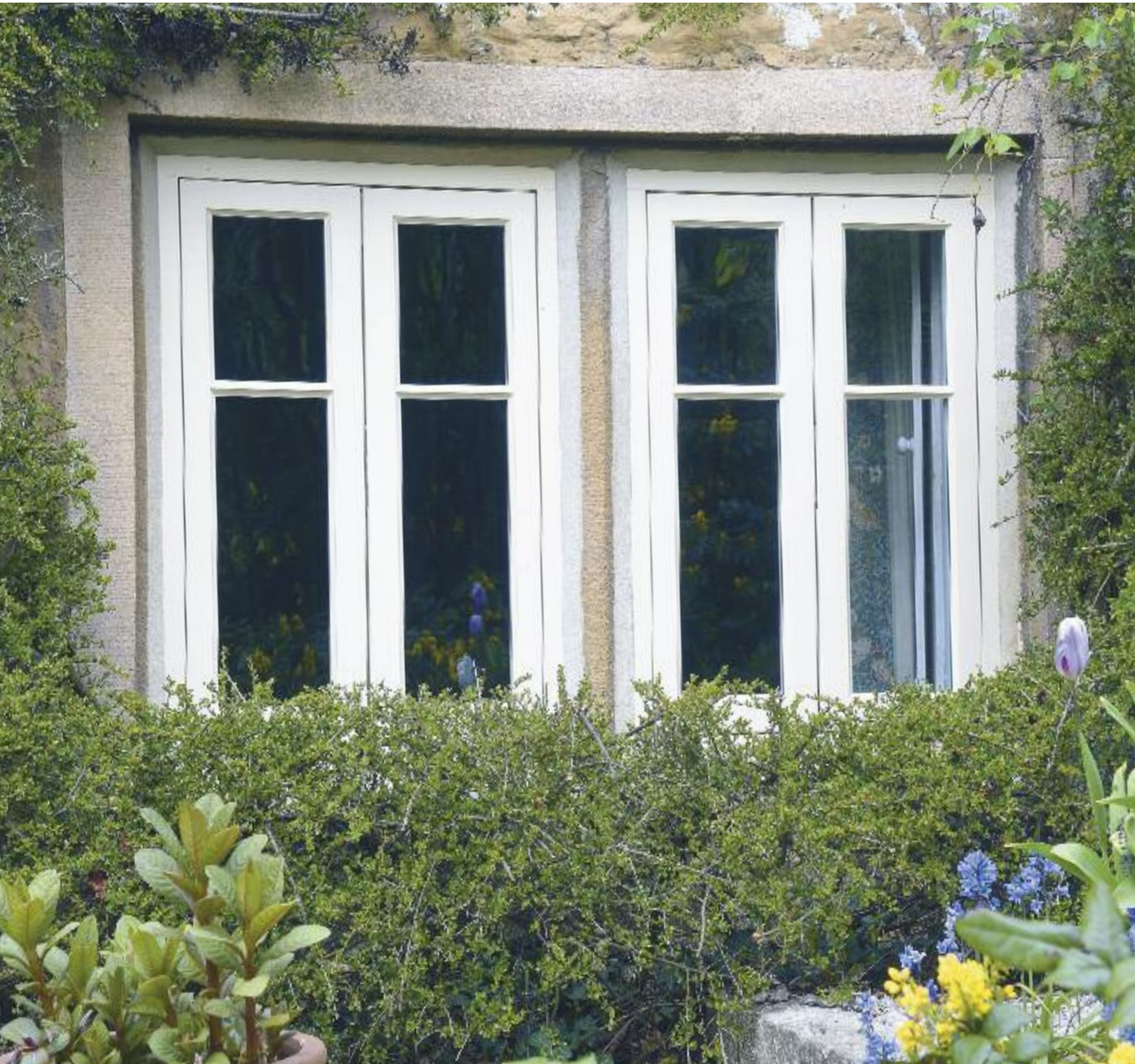
Cottage flush casement windows featuring 14mm ultra slim double glazed units with krypton gas, 22mm true bars and putty glazing, externally finished in the shade of 'Dorset Cream' and internally in 'White'.
